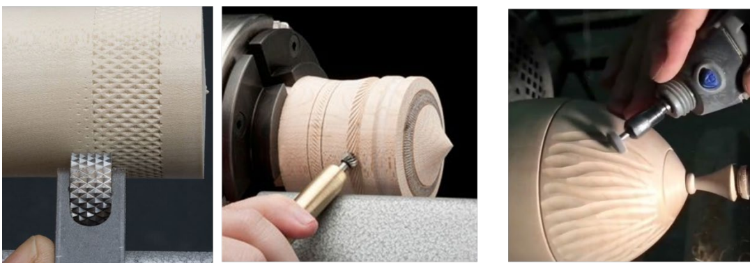
Examples of on-lathe applied texturing.
